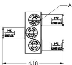
REMOVALBE CAPS FOR ACCESS TO 3/16 INTERNAL HEX PRESSURE SCREWS
