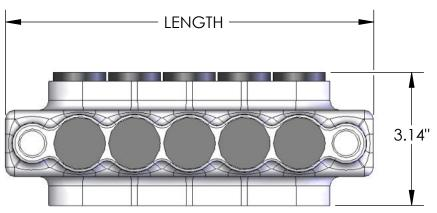
INSULATED MOUNTING PORT ON EACH END FOR A 5/16 BOLT
