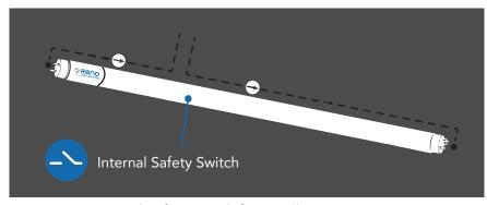
Internal Safety Switch for installation protection. (No curent will flow until pins on both ends are engaged)
