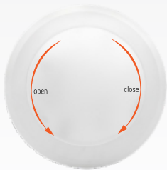
Anticlockwise to open the outside lens
