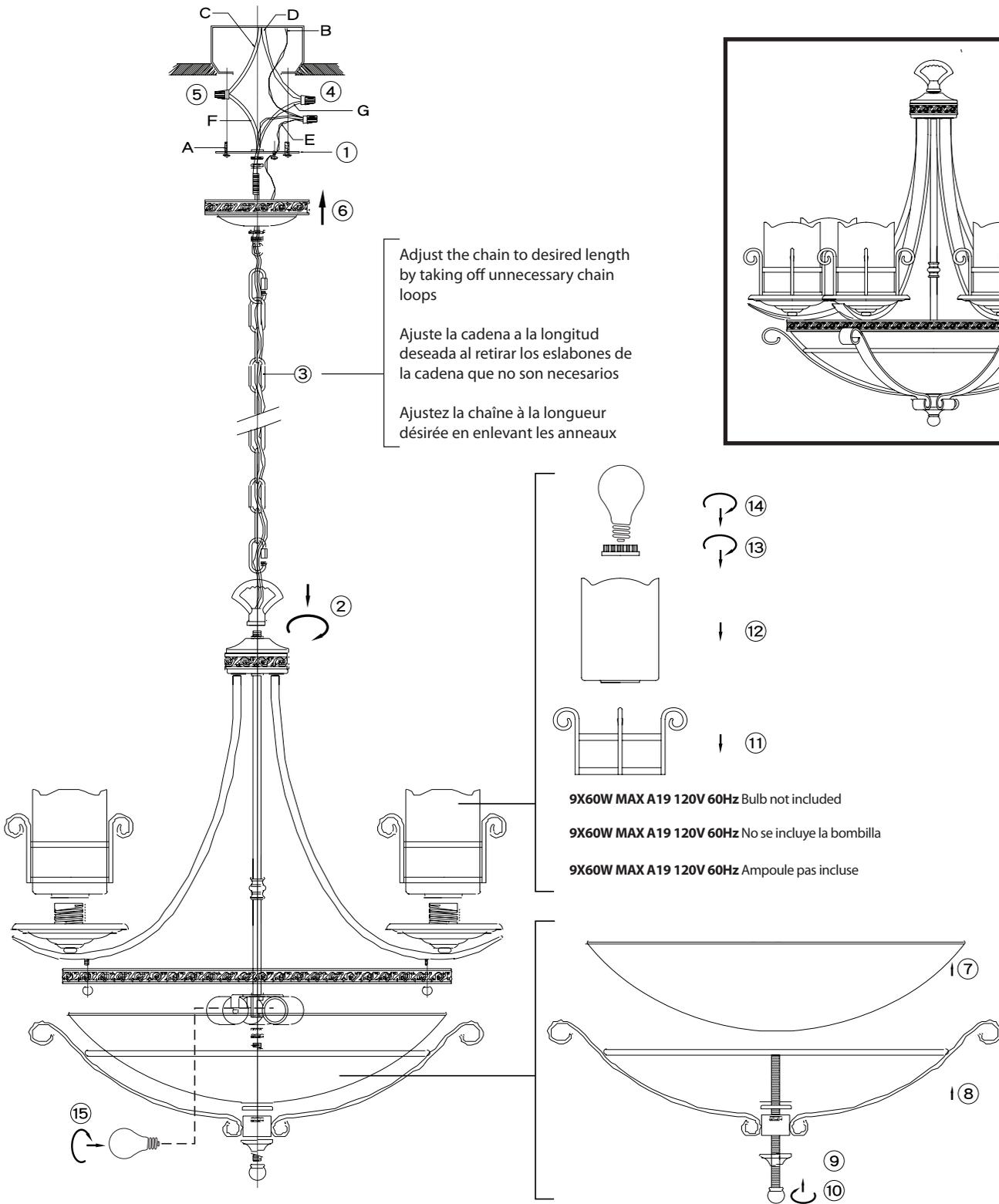
Adjust the chain to desired length by taking off unnecessary chain loops
