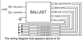
The wiring diagram that appears above is to the lamp type denoted by the asterisk (\*)
